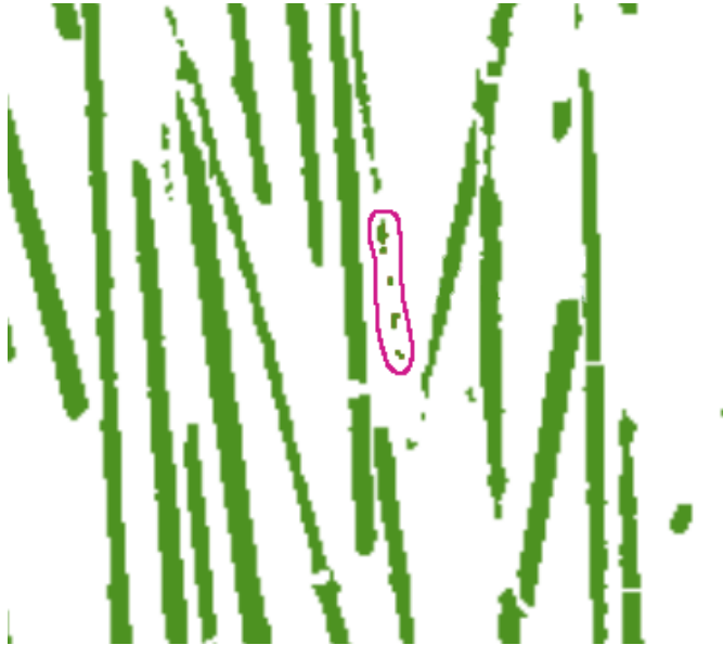
Figure 5.12: Cutout of the XZ-slice 170 of the GFRP dataset before enabling the fish-eye lens. The focus is on the pink circled fibre parts.
