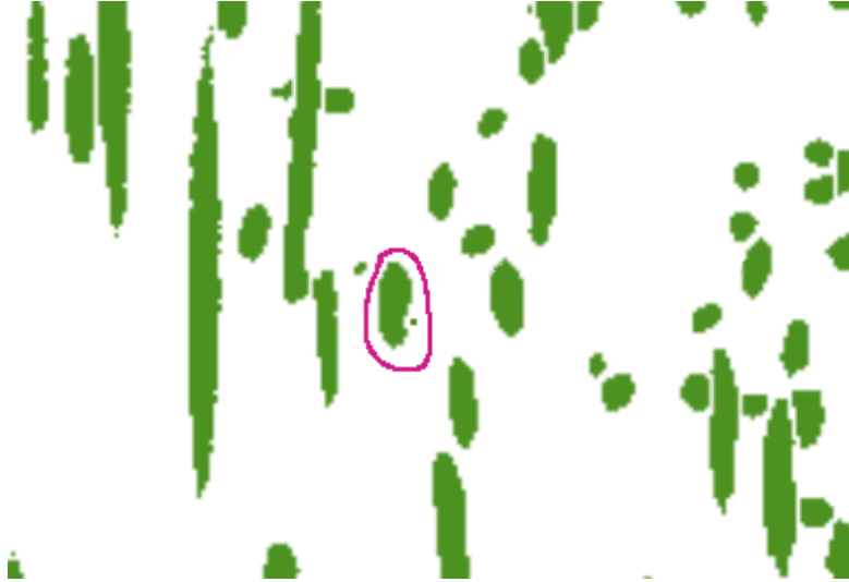
Figure 5.10: Cutout of the YZ-slice 199 of the GFRP dataset before enabling the fish-eye lens. The tiny fibre part to the right inside the pink marked circle is going to be magnified.
