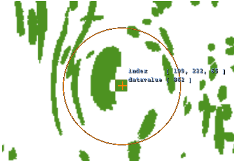
Figure 5.11: Cutout of the YZ-slice 199 of the GFRP dataset with fish-eye lens magnification.
